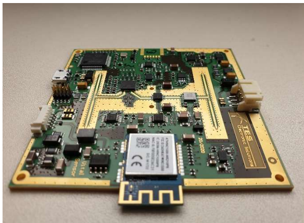
Fig. 1 The top layer view of the PCB of the TES Vital Radar Sensor (left). The bottom layer view of the TES Vital Radar Sensor PCB showing the patch antenna with the PCB mounted on an Aluminum casing (right).
