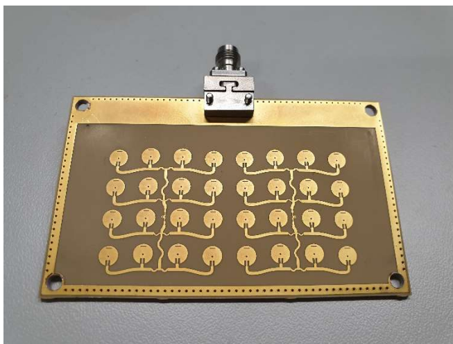
Fig. 1 The 8 \times 4 planar antenna array fitted with an RF connector for signal feed-in (left). Two copies of the 8 \times 4 planar antenna array (i.e. for transmitter and receiver) used together for a radar application (right).
